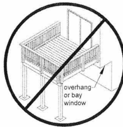
Figure 18: No Attachment to House Overhang
